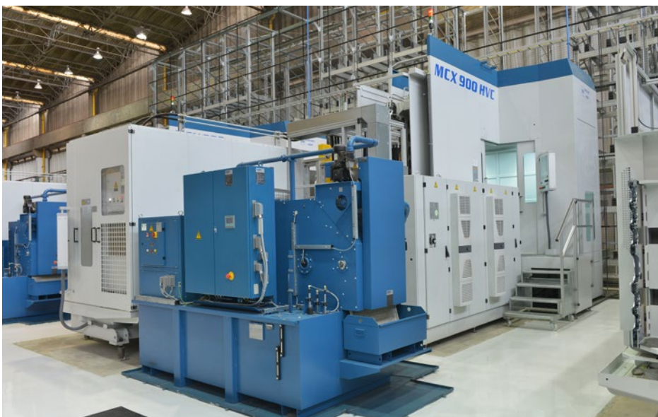
MCX 900 integrated in Fastems storage system
