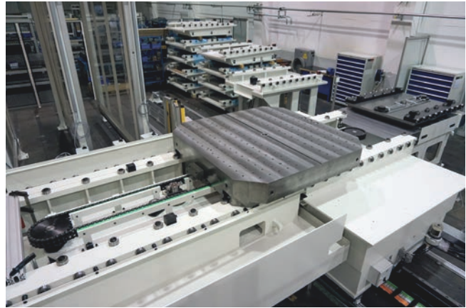
Transfer of a workpiece pallet from the tooling station to the pallet transport vehicle
