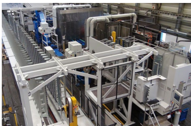
In the foreground: the transfer shuttle.
