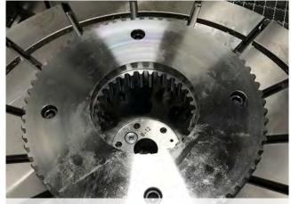
Machined component, internal and external ring gears, up to a diameter of 2,800 mm / module 8 (depending on tool).
