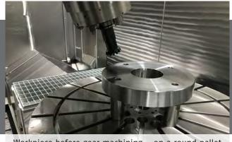
Workpiece before gear machining – on a round pallet with T-slots.
