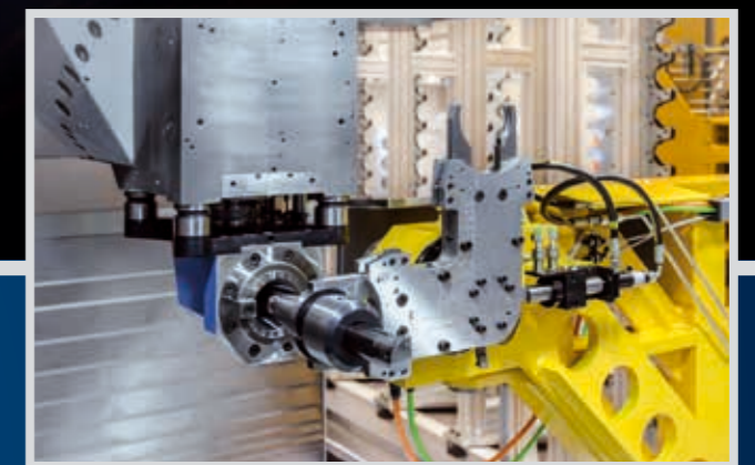
Automatic exchange of turn-tool holder in turn-tool adapter.
