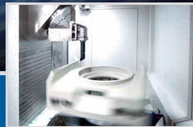
Robustly dimensioned tilting spindle with quadruple turn-tool holder clamping. Automatic changing of all turning tools from the standard magazine.
