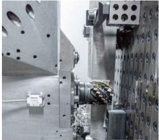
3 As part of testing to produce slots using a five-bladed 80-mm sprocket cutter, there were machining processes with virtually no measurable vibrations (© Burkhardt+Weber)
