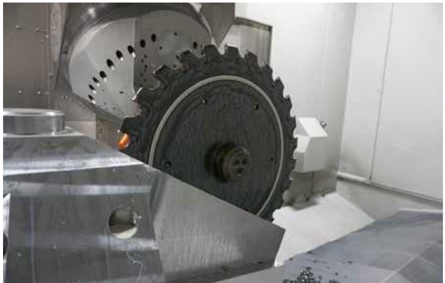
1 Heavy machining in action: A 600-mm side milling cutter works on an HVC head on a Burkhardt+Weber machining centre. The tool requires that the machine has an extremely high torque in the lowest speed range (© Burkhardt+Weber)
